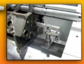
CWT's Exclusive Mounting System allows blocks with and without Cam Bores to be quickly mounted. Also eliminates special clamps when honing OHC Cylinder Heads.
