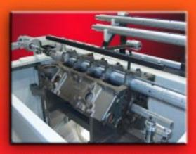
Aluminum Diverter is used to direct all oil and waste materials to a magnetic pre-filter and then directed to the 20 Gal. removable reservoir, followed by sending the fluid to our twin filter pump system.
