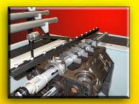
Oil Flow is controlled by a series of needle and seat valves, This allows the technician to apply oil directly to each Main Bearing.
