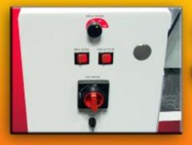
Operator Control Panel allows quick access to speed controls and On/ Off switches. Available in 120/240 volts, 50/60 Hz.
